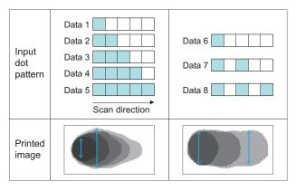
Figure 3 Example of obtaining the parameter for dot pattern simulation. Line width and line length change depending on variable input data patterns.
