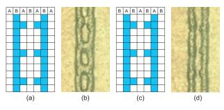
Figure 6 Differences of coverage depending on a differences of dot placement order. (a) (c) indicate input images and (b), (d) indicate printed results. Data for column A is printed before data for column B is printed.
